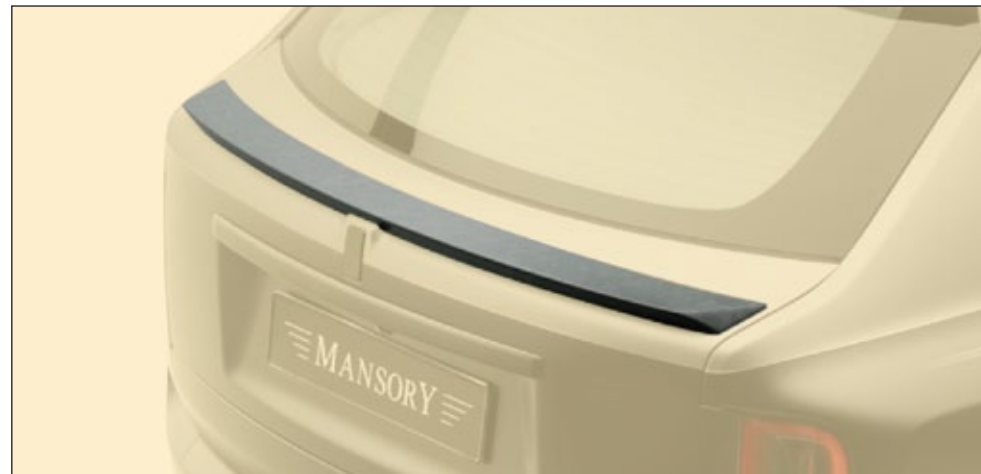
Rear decklid spoiler - exposed ..... RRC 830 841 visible carbon fibre primed without clear coat
